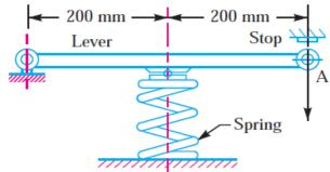
Assuming a spring index as 8, determine: 1. spring rate, 2 size of wire, 3. outside diameter of the spring, 4. number of active coils, and 5. free length, assuming squared and ground ends. The allowable shear stress may be taken as 420 MPa and  $G = 80 \text{ kN/mm}^2$ .
