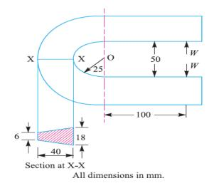
2 The crank hook carries a load of 20 KN as shown in FIG.(2). This section at X-X is rectangular whose horizontal side is 100mm. Find the stresses in the inner and outer fibers at the given section
