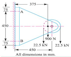
2. A wall bracket, as shown in Fig. 11.50, is fixed to a wall by means of four bolts. Find the size of the bolts and the width of bracket. The safe stress in tension for the bolt and bracket may be assumed as 70 MPa.
