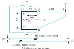
10. A bracket, as shown in Fig. 10.39, carries a load of 40 kN. Calculate the size of weld, if the allowable shear stress is not to exceed 80 MPa.
